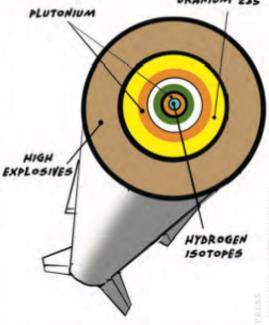
CREATING A NUCLEAR EXPLOSION IS NOT EASY. IT RE-CONVENTIONAL EXPLOSIVES. THE SUDDEN COMPRESSION OF THE TWO FISSILE ELEMENTS CREATES A CRITICAL MASS, STARTING A CHAIN REACTION RELEASING MASSIVE AMOUNTS OF ENERGY. IN BOOSTED FISSION, HYDROGEN MOLECULES ARE PLACED IN THE FISSILE CORE, INCREASING THE PRESSURE AND TEMPERATURE, ACCELERATING FISSION.
